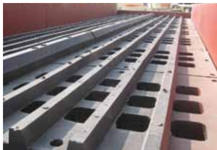
Panelcord equipment (primary CVB screen)
